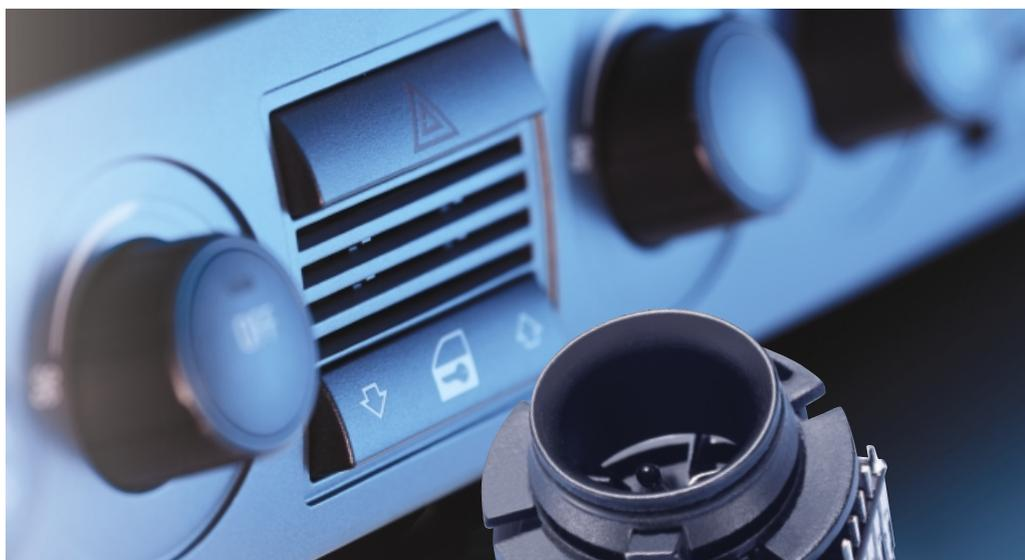
In the climate or roof control units of many makes of vehicle, sensor blowers accurately detect the interior temperature of the vehicle. Alternative variants of these tiny blowers, equipped with independent operating electronics, can also be used at any desired location in the instrument panel or rear passenger area.
