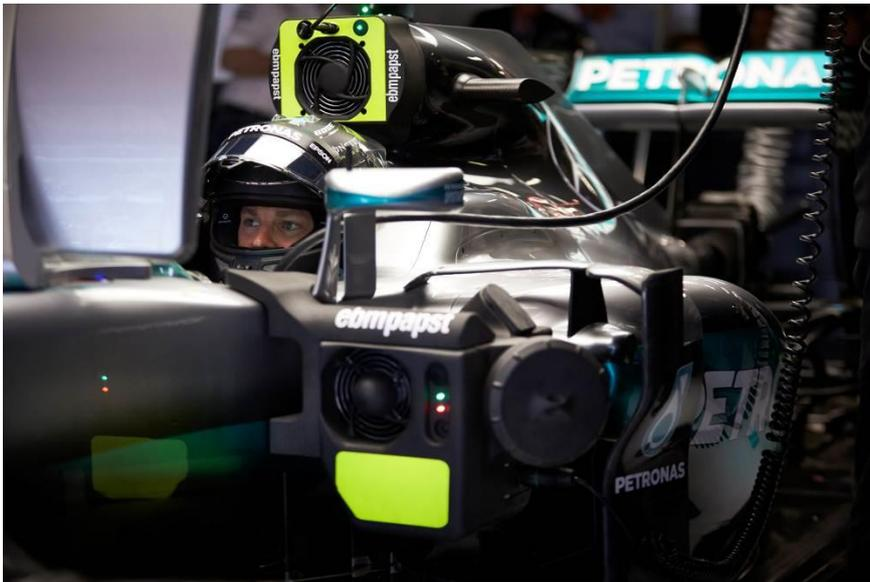
Photo 1: A cooling system devised by ebm-papst conveys trapped heat out of the openings in the side-pods and the roll-hoop.
