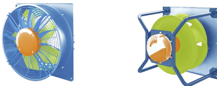
Figure 3: The central functional areas of axial (left) and centrifugal fans (right): the impeller as the aerodynamic core (green), the motor with integrated electronics as the drive unit (orange) and the stator , i.e., the air-conducting and supporting structures (blue).
