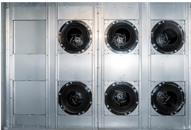
Fig. 2b: If one of the fans fails, the speed of the others is increased so that the air performance always remains the same. This makes this solution particularly reliable for critical applications.
