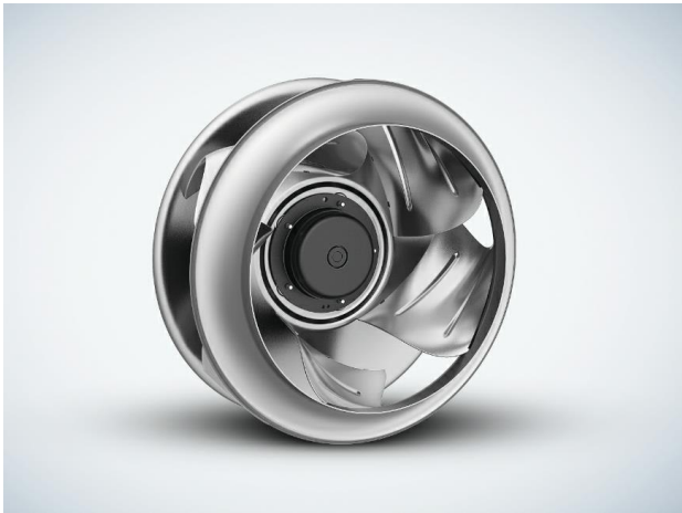
Fig. 1: RadiPac EC centrifugal fans from ebm-papst are specially designed for filter-fan-units in cleanrooms. The newly developed impeller with its five geometrically sophisticated impeller blades drastically reduces flow losses.
