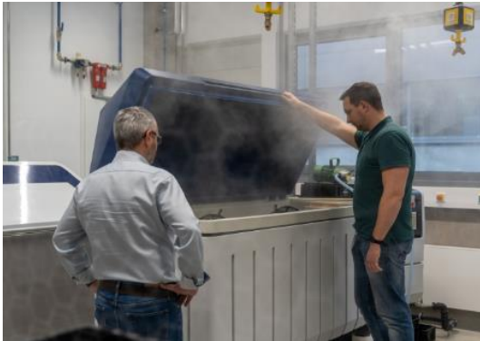
Image 4: The quality of the coatings and materials is investigated in the salt spray test chamber.
