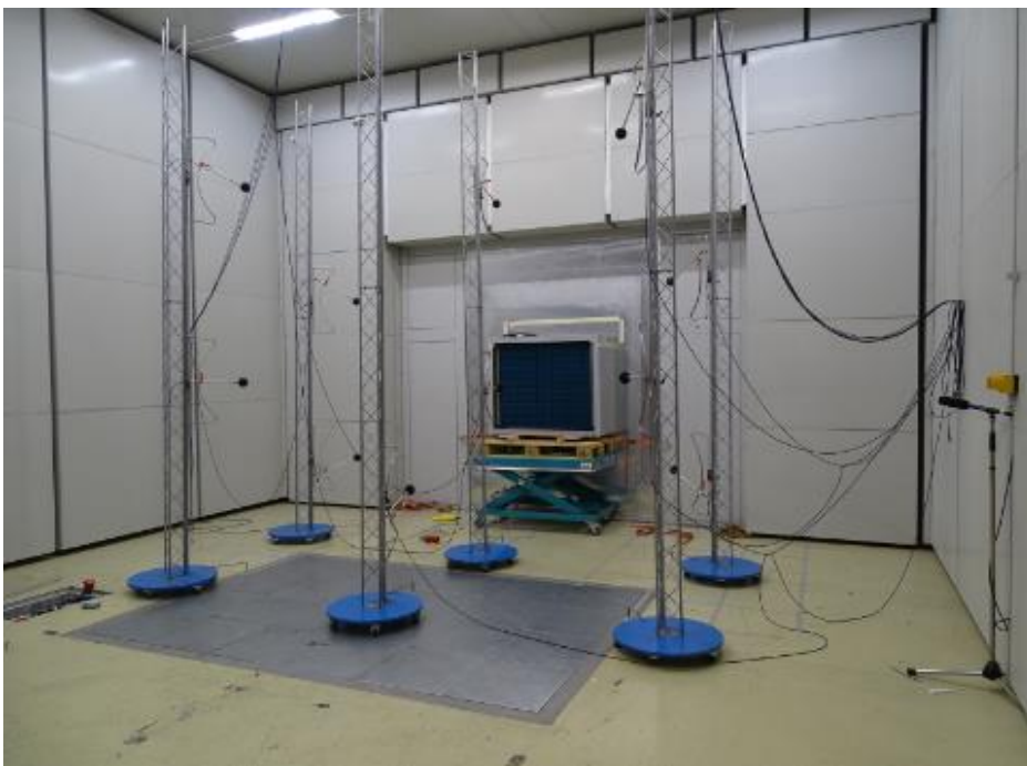
Fig. 2: In the ebm-papst test facilities, heat pumps together with the fans installed in them are recorded aerodynamically and acoustically.
