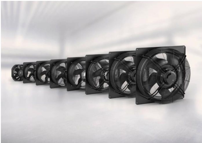
Figure: The AxiEco series has been expanded to include three new larger sizes, which means that air flows of over 25,000 m 3 /h and pressures of up to 700 Pa can now be achieved.
