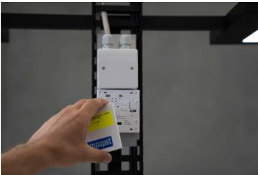
Fig. 2: The certified sensors constantly measure the air quality and send their data to ebm-papst's cloud-based Building Connect platform, which processes it further.
