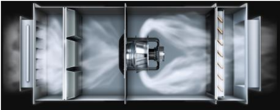
Fig. 1: Flaps and filters can obstruct the air flow in AHUs, and the distance to walls and heat exchangers as well as the use of guard grilles also have an effect – which is why the actual installation situation must be considered at an early stage to achieve an optimal result at the end of development.
