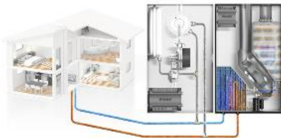
Fig. 2: The higher-level control system – the 900H Series Control Platform from ebm-papst – controls the output of the gas condensing unit and heat pump, based on the situation.
