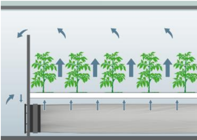
Picture 3: With ventilation tubes, the air is supplied underneath the plants, providing an optimum supply of CO 2 to the undersides of their leaves.
