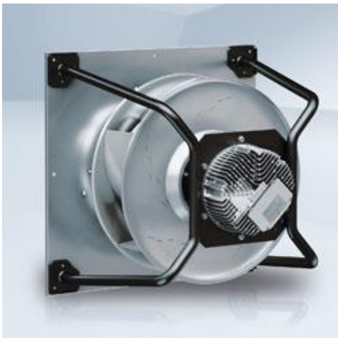
Fig. 2: In shipbuilding, every cubic centimeter counts. In RadiPac EC fans, the high-performance impeller is directly attached to the rotor of the external rotor motor, making the system extremely compact.
