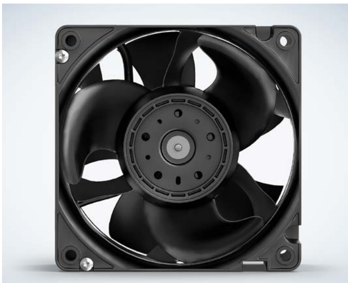
FIGURE 3: Second-stage fan impeller: turbulence and swirl are reduced. The blade's extreme sickle shape also contributes to noise reduction; the comparatively small surface of the blades increases efficiency.
