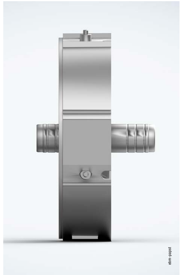
FIGURE 4: The flange is more than a spacer. Thanks to its optimized geometry, it reduces the generation of vortices and noise at the second stage.
