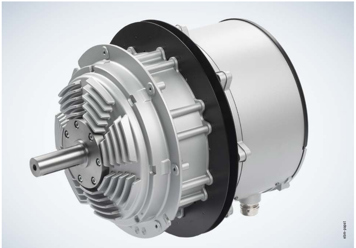
FIGURE 1: Powerful EC motor with external rotor design. With outputs of up to 24 kW and a torque of up to 180 Nm, it is suitable for universal use on large fans.
