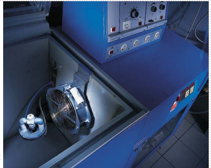
FIGURE 6: Fans often have to withstand harsh ambient conditions and therefore pass through various test stations beforehand, such as the salt spray test at ebm-papst.
