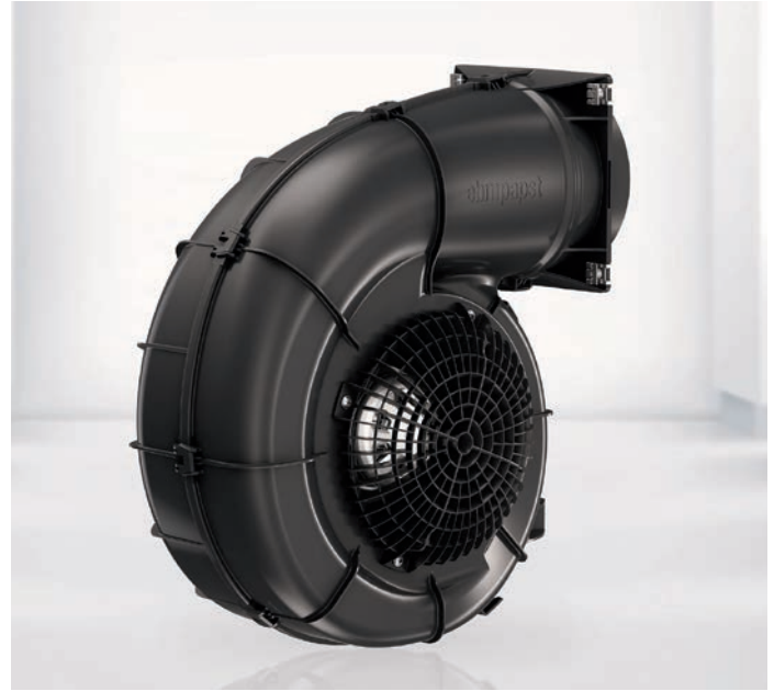
FIGURE 3: The latest generation of EC centrifugal fans, the RadiCal with vane anemometer for independent air flow measurement and regulation, backward-curved, single inlet with housing (flange).
