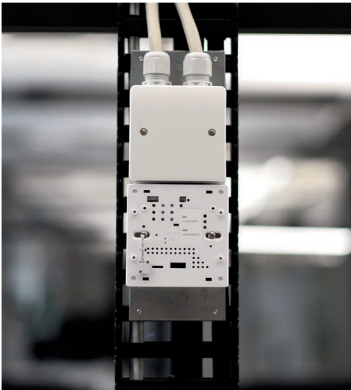
FIGURE 5: The sensors, which are certified according to the only real-time-based, internationally recognized air quality standard for indoor spaces, RESET, continuously measure the air quality and send their data to ebm-papst's cloud-based Building Connect platform, which processes it.
