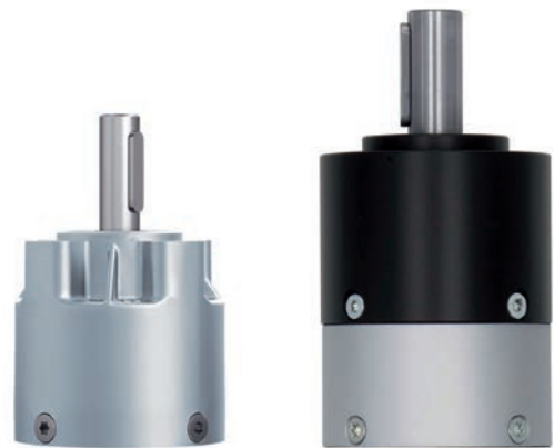
FIGURE 2: Due to greater tooth widths in the input stage and the increased strength of the ring gear toothing made of hardened steel in the output stage, the PerformaxPlus planetary gear is particularly suitable for high torques.
