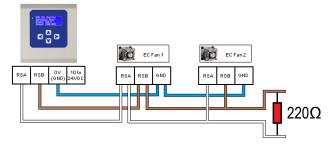
In case the controller is in the middle of the network, the built-in termination resistor must be taken out of the circuit by removing the jumper bar located on back of the PCB. If that is the case, two resistors of the same value must be added at each end of the network.
