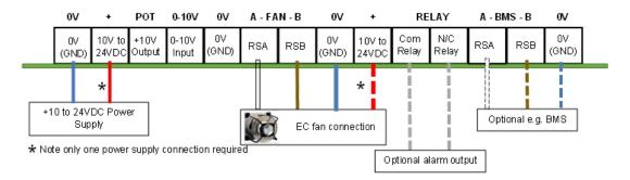
⚠ CAUTION: Danger of damaging the fan if two different power supplies are connected at the same time
