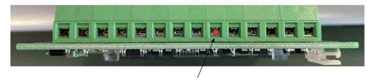
Sealing Plug: <u>DO NOT CONNECT the 10VDC</u> output from fans here if the controller is powered from an external power supply.
