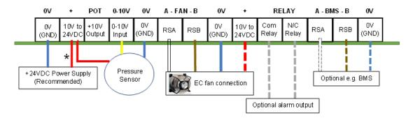
Alternatively, it is possible to connect the pressure sensor to the fan's 0-10V input - for more information please read the full operating and maintenance instructions document identify 210-OMI14229.
