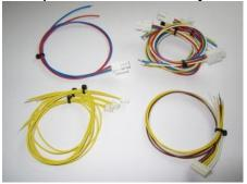
Development Cable Set Accessory ebm-papst part number 210-HAR13100. This consists of a TMS power cable, 4 off fan cables, alarm cable and switch input cables. The cables consist of the required mating connector for the TMS connection, the other end of the cable being unterminated to allow the user to connect as they require. This is intended for development or evaluation use, particularly by customers that do not have tools to fit the necessary connector crimps.
