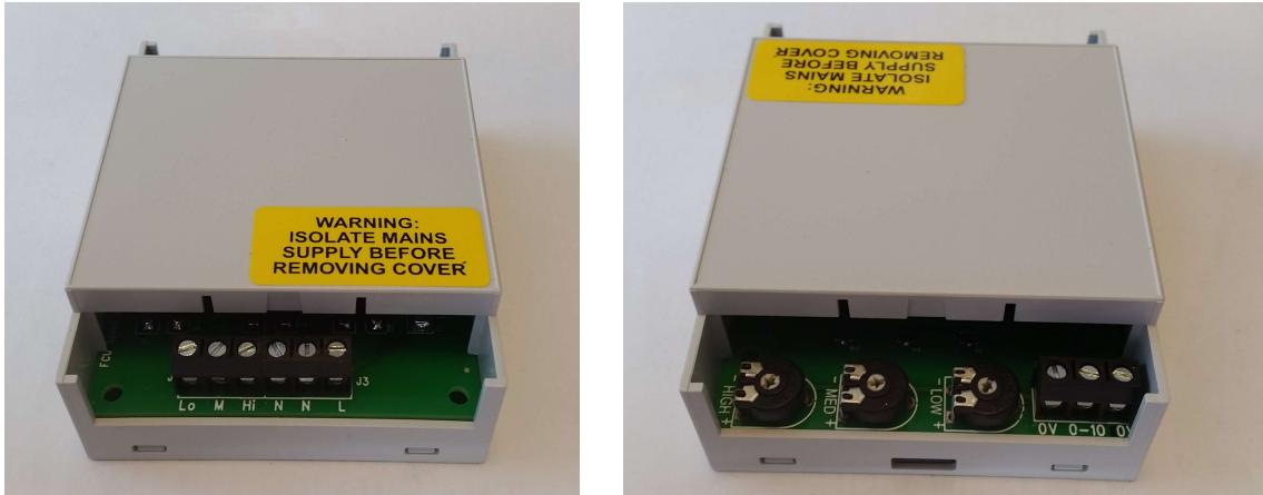
Figure 2 - Mains and control connections
