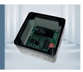
The RM-ECd controller is for use with the full range of ebm-papst EC fans. Powered by the 10VDC output from the motor, it provides infinitely variable, manual speed control between 0% and 100%. The control voltage 0-10v is displayed on the LCD for ease of commissioning. A DIP switch allows display of rpm instead if a tacho fan is used.
