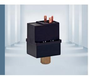
These two pressure sensor speed control devices are for refrigeration pressure control applications. The 0-10 V DC signal output is proportional to the refrigerant pressure. The output can be connected directly to ebm-papst EC fans providing a closed loop control.
