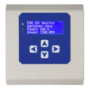
The Modbus Display & Control (MDC) is a device with two RS485 Modbus ports, a keypad for setting parameters / navigating and a display to view the status of the connected fans. The RS485 Master port connects to up to 100 Modbus EC fans and the RS485 Slave port allows an interface to a higher-level Modbus Master device e.g. BMS or IoT dataloggers if required. The MDC has its own "fan auto-addressing" feature to ease installation and commissioning, and supports four different operating modes.
