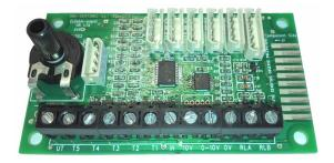
Primarily designed for use with our EC fan coil fans. This provides a simple and low cost monitoring solution for up to 5 EC fans per board, with fan alarm relay output, and LED to identify failed fan.
