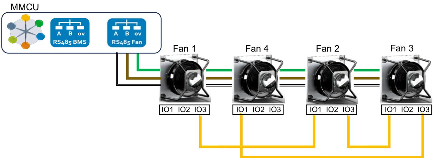
Figure 3 – Daisy chain reordering extra fan connection
