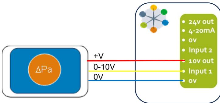
Figure 5 – Example pressure sensor connection to controller
