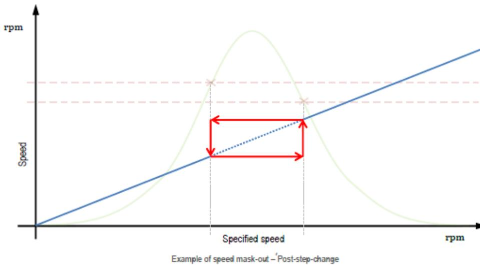
Figure 19 - Resonance avoidance speed mask post-step change
