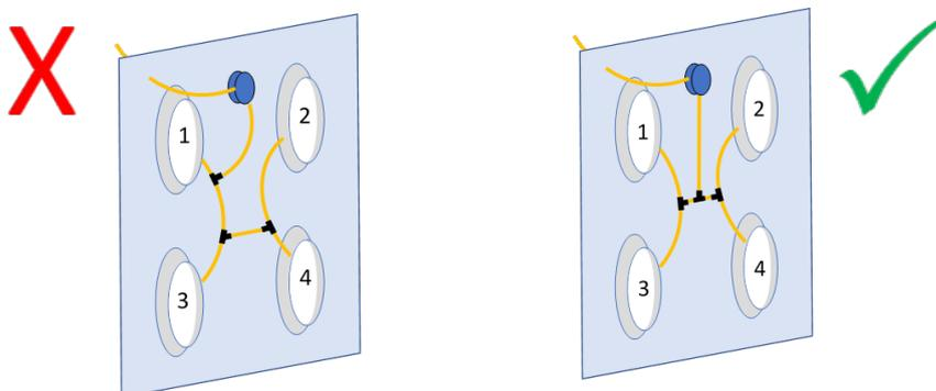
Figure 10 - Connecting to tapping rings for Volume measurement.
