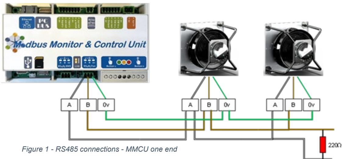
Figure 1 - RS485 connections - MMCU one end
