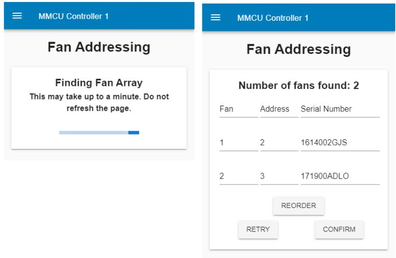
If after 1 minute the controller cannot find an existing array of fans it will advise to check the network wiring and power and then return to the addressing menu to try again.
