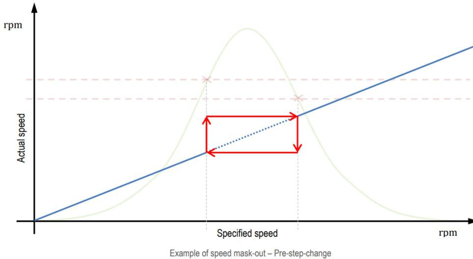
Figure 18 - Resonance avoidance speed mask pre-step change
