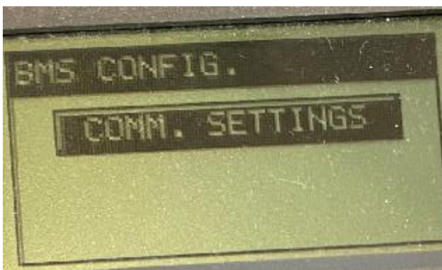
Figure 20: Gateway screen - set Ethernet TCP/IP communication parameters
