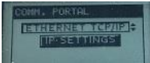
Figure 22: Gateway screen - set Ethernet TCP/IP communication parameters
