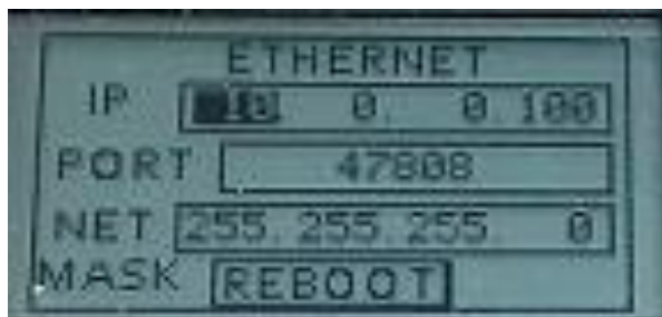
Figure 23: Gateway screen - set Ethernet TCP/IP communication parameters
