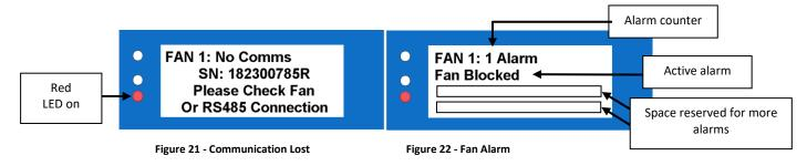
If a fan has more than one alarm, they will be displayed in a list as they occur, and the alarm counter will increment. The controller's screen can display up to 3 fan alarms per fan.
