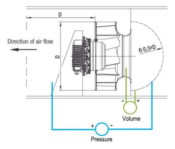
Figure 14 – Sensor airline connections for pressure and volume
