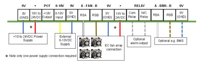
Figure 10 - Wiring diagram for Monitor & Control operating mode and 0-10V control mode – external control signal
