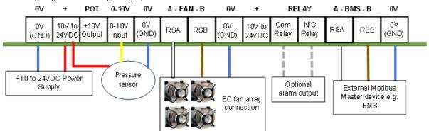
Figure 13 - Typical wiring diagram for Constant volume / Constant pressure operating mode and controller sensor input
