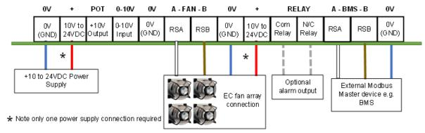
Figure 11 - Wiring diagram for Monitor & Control operating mode - Modbus RS485 control signal
