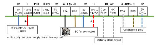
Figure 2 - Typical wiring for Monitor Operating mode
