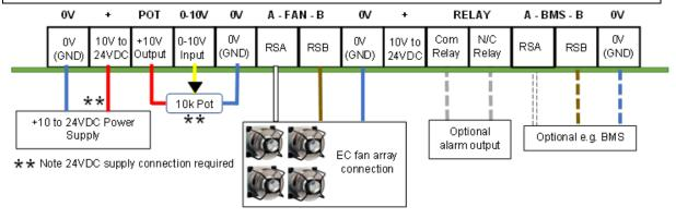
Figure 9 - Wiring diagram for Monitor & Control operating mode and 0-10V control mode – potentiometer control signal and external power supply
