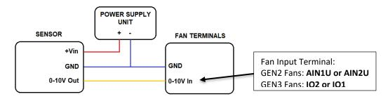
Figure 16 - Sensor-Fan wiring diagram with power supply
