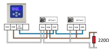
Figure 1 - Schematic of RS485 installation
