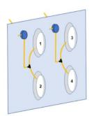
Figure 18 - Example of sensor airline connections in a 4-fan 2-sensors constant volume system
