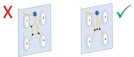
Figure 15 – Airline length for a single sensor constant volume system or volume monitoring system
