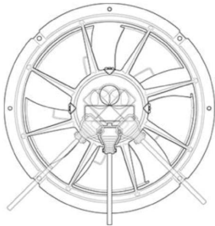
Fig. 2: Cable routing for fans installed upright.
