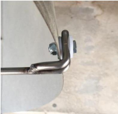
*Nut, metal washer, diffuser pieces, nylon washer, guard grille, nylon washer and then the bolt.*
