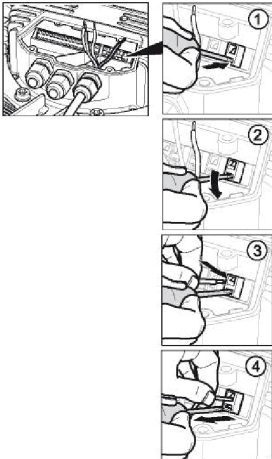
Fig. 2: Connecting the wires to the terminals.
