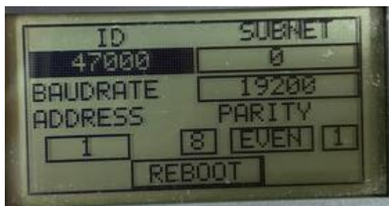
Figure 31: Gateway screen - set MS/TP RS485 communication parameter
