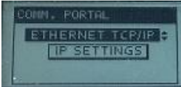
Figure 21: Gateway screen - set Ethernet TCP/IP communication parameters
