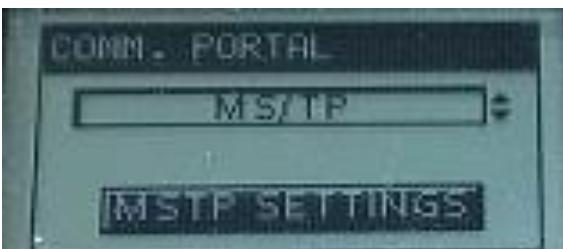
Figure 30: Gateway screen - set MS/TP RS485 communication parameter
