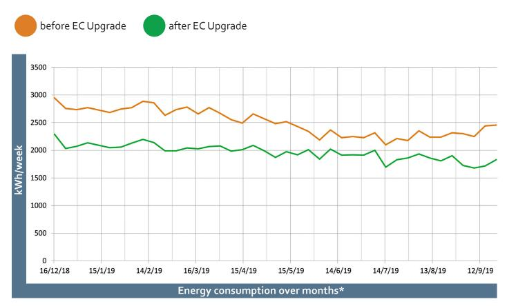
\* Medium temperature rack power consumption includes: compressors & condenser fans
