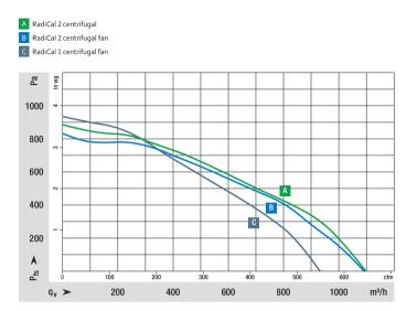
The RadiCal 2 outperforms its predecessor with high air flow rates. The new centrifugal module is now slightly above the motorized impeller.
