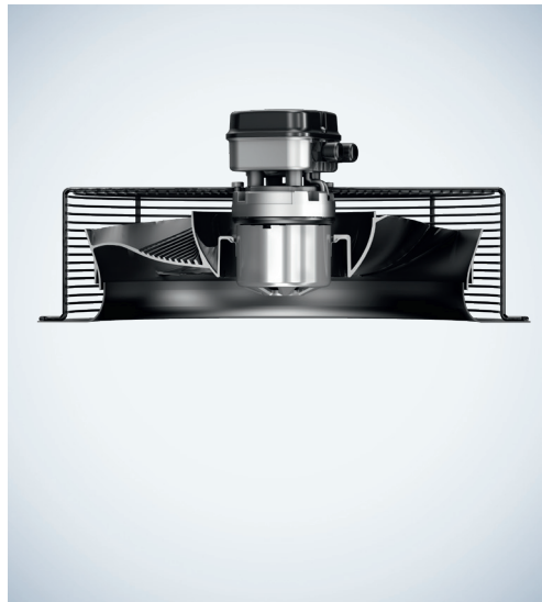
Fig. 6: The fan has an optimal throughflow thanks to the inlet ring that immerses in the impeller and thanks to the impeller's larger outlet opening.
