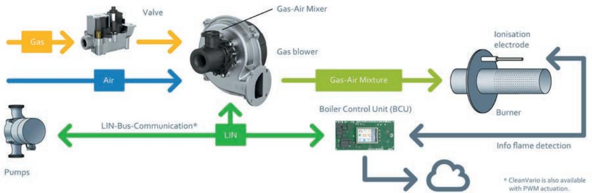
FIGURE 3: CleanEco pneumatic combustion control (top) and CleanVario electronic combustion control (bottom) offer a perfectly coordinated complete system consisting of a boiler control unit (BCU), gas valve, Venturi and gas blower.
