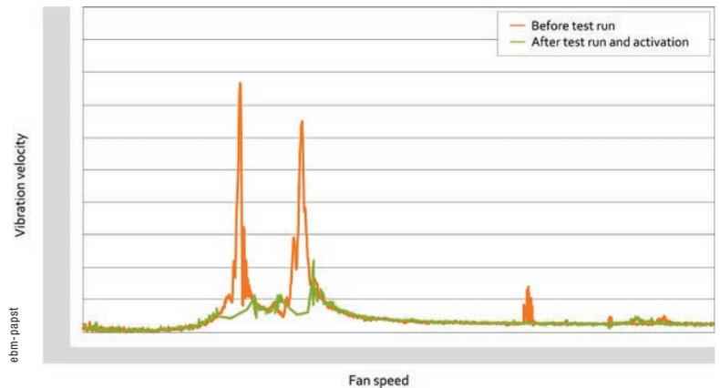
FIGURE 6: If standard resonance detection is activated, ranges with excessive vibration velocities are detected and “overrun”.
