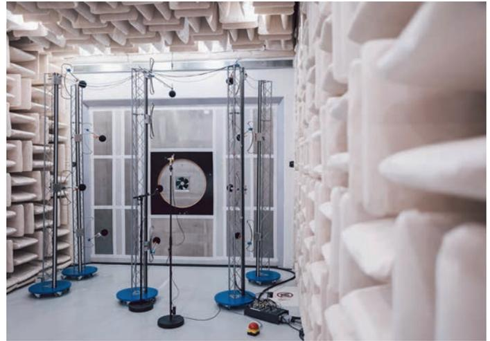
FIGURE 3: The data sheet specifications are determined on the test stand. These must be based on reproducible measurements under (un-disturbed) standard conditions.
