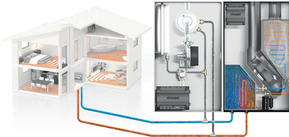
FIGURE 4: The 900H Series Control Platform from ebm-papst adapts the output of the hybrid system according to the situation, and controls the connection of the condensing boiler when temperatures drop below zero.
