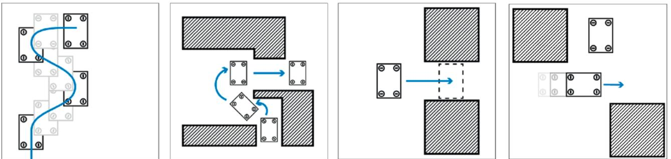
FIGURE 2: With the ArgoDrive driving/steering system from ebm-papst, AGVs navigate freely and omnidirectionally over the entire area, drive around unexpected obstacles and move easily even in very tight environments.
