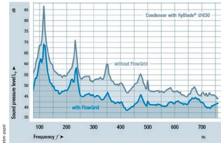
FIGURE 7: Additional parts such as the FlowGrid can also be used to reduce unpleasant effects after installation.
