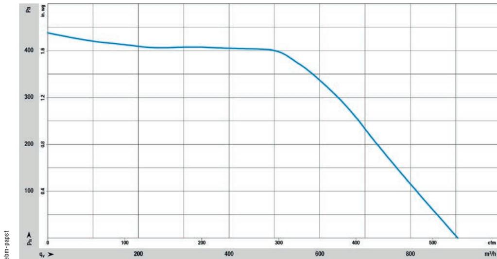
BILD 2: Good performance: The RadiFlex can move up to 930 cubic meters of air per hour (free air).
