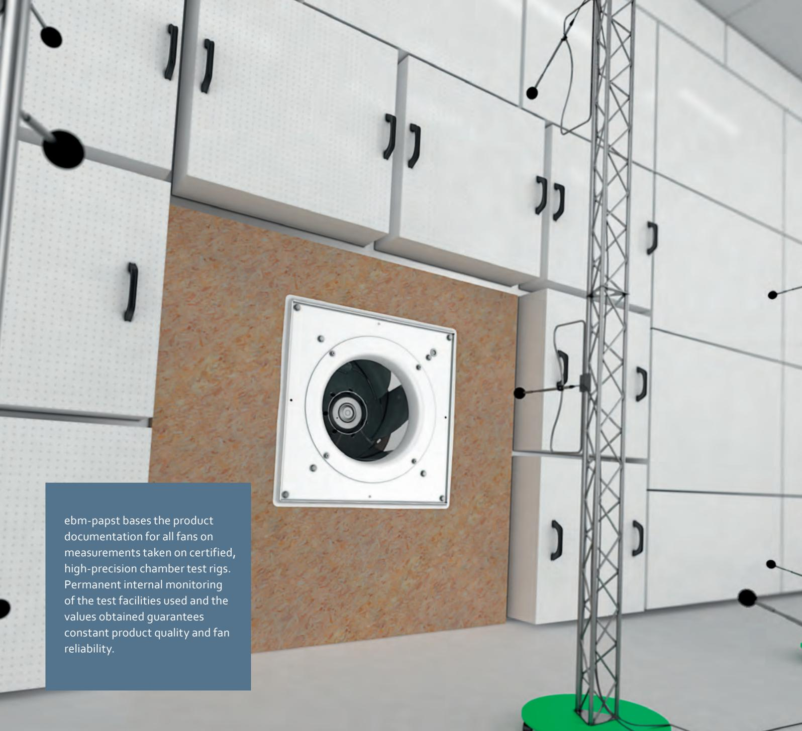
ebm-papst bases the product documentation for all fans on measurements taken on certified, high-precision chamber test rigs. Permanent internal monitoring of the test facilities used and the values obtained guarantees constant product quality and fan reliability.
