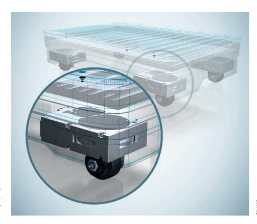
FIGURE 3: A new drive solution for AGVs with free-range mobility: The ArgoDrive driving/steering system from ebm-papst. with high maneuverability, such as the Mecanum wheel, quickly run into problems here, because they require smooth ground to move. However, this restriction is not necessary, as there are driving/steering systems that meet all the requirements of future-proof AGVs.
