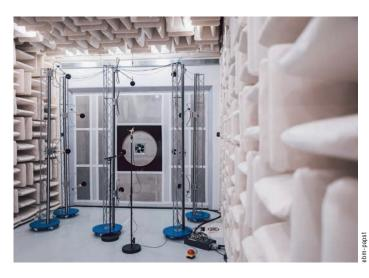
FIGURE 3: The data sheet specifications are determined on the test stand. These must be based on reproducible measurements under (undisturbed) standard conditions.
