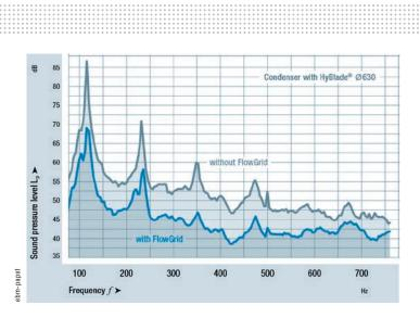
FIGURE 7: Additional parts such as the FlowGrid can also be used to reduce unpleasant effects after installation.
