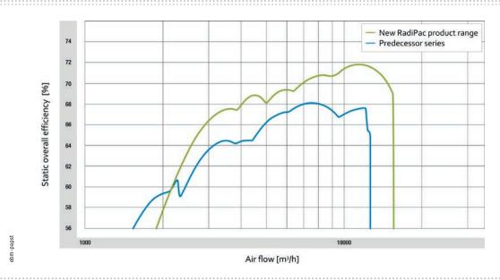
FIGURE 1: The new Radi-Pac: The new generation of centrifugal fans offers higher efficiency; this results in significantly lower operating costs.
