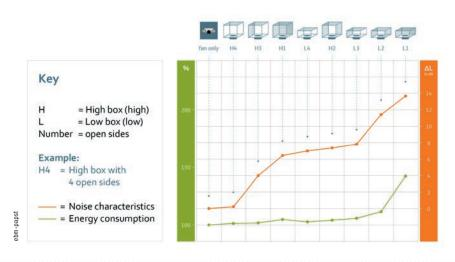
FIGURE 4: Energy consumption and noise change, depending on how the housing influences the flow – i.e. whether it is drawn in axially from the front, centrifugally from all sides, or on one side.
