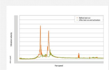
FIGURE 6: If standard resonance detection is activated, ranges with excessive vibration velocities are detected and "overrun".
