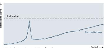
Fig. 1: Vibration characteristics of the fan
