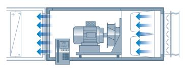
AC fans (AC standard motor with variable frequency drive)
