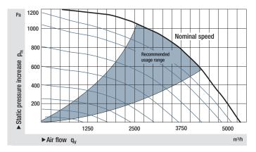
Characteristic curve of a centrifugal fan with a broad useful range.
