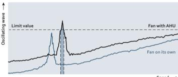
Fig. 3: Vibration behavior with speed range that has been omitted
