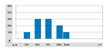
For the given load profile, the GreenTech EC fans has an advantage of roughly 28% over a standard AC fan of the same power with variable frequency drive.
