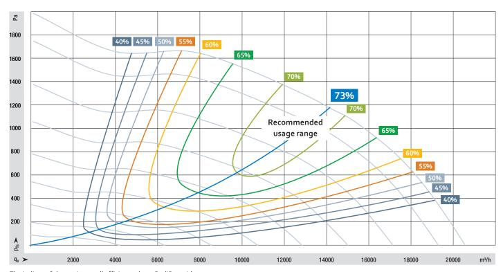
The isolines of the static overall efficiency show: RadiPac with broad, efficient usage range. Furthermore, they provide information about the efficiency levels in partial-load operation.
