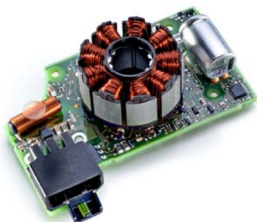
Figure 2: BLDC motor with outer rotor for urea pumps
