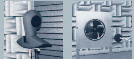
Room for precision noise measuring
