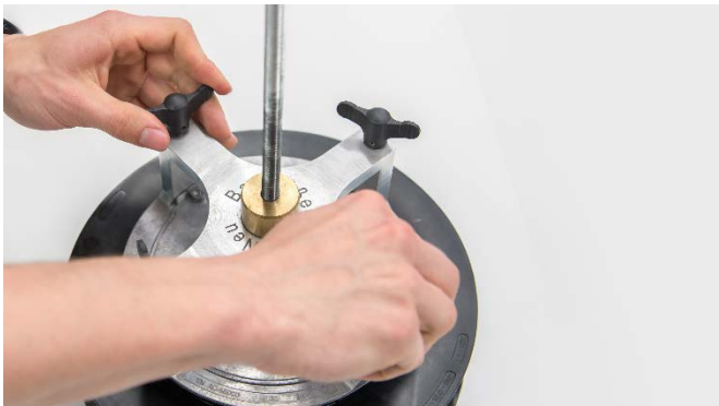
12. Fit the puller and screw it in position at all four tapped holes in the stator.
