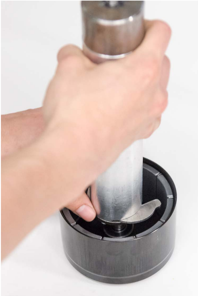
17. Position the puller in the center and screw it on.
