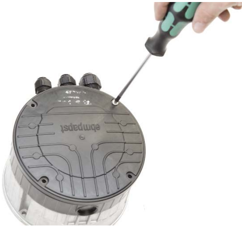
a. Unfasten the four screws at the plastic terminal box and detach the cover.
