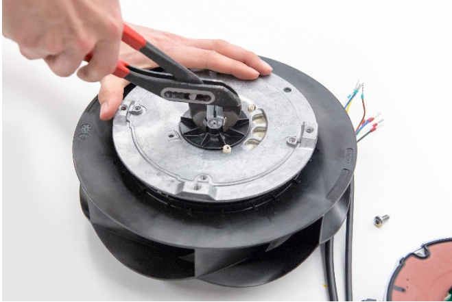
10. Use water pump pliers to detach the small fan impeller.
