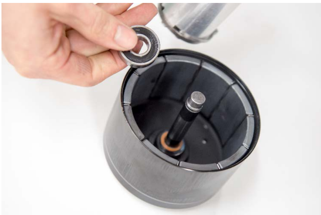
19. Take the ball bearing out of the puller and remove the two washers from the rotor bell.
