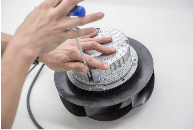
1. Unfasten the four screws at the housing.
