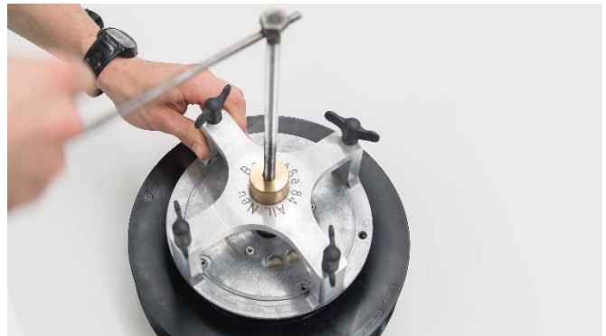
13. Unfasten the stator by turning the spindle in the puller in clockwise direction.
