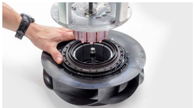
14. Lift out the stator with the puller. Then remove the puller again.
