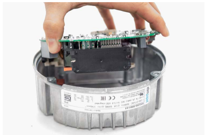
9. Completely remove the circuit board.
