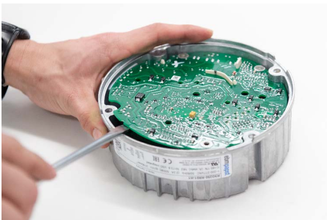
8. Use a screwdriver to prise out the circuit board.
